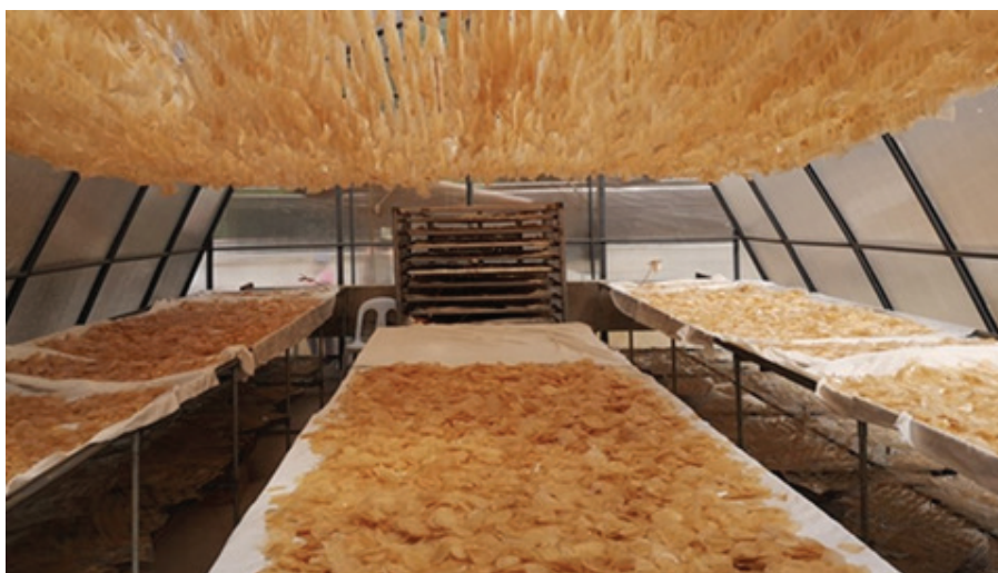
Figure 4.1. Greenhouse solar dryer installed and tested in Dapitan, Zamboanga del Norte
