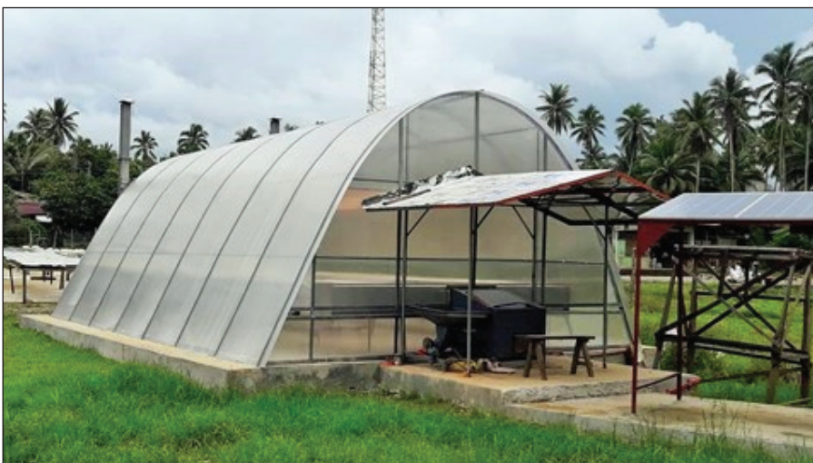
Figure 4.2. Greenhouse solar dryer installed and tested in Naguilian, Isabela
